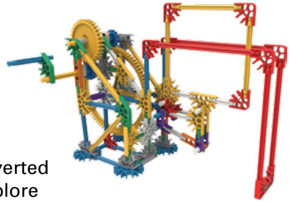
**Objectives:** Observe how rotational motion is converted into linear motion using a spur gear system and explore spur gears as a means to multiplying output force.
