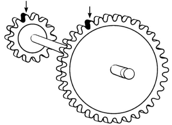
(i) Turn the blue crank through 1 full turn and notice how far the tan and yellow gears turn. You can count the number of teeth the gear moves through, or you may want to consider the movement in terms of the hands on the clock. For example the gear moves from 9 o'clock to 2 o'clock. You should record your answers in a table such the one shown below.
